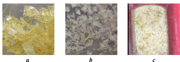
Figure 1. Polysiloxane-urea after separation from the reaction products (a), ground polysiloxane-urea (b), polysiloxane-urea which was loaded into the extruder hopper (c).
