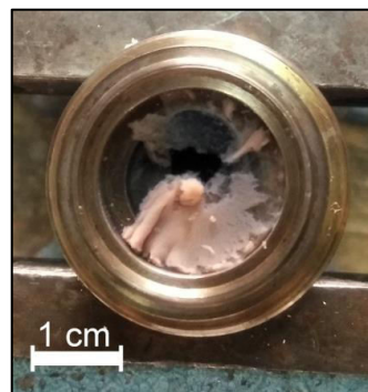
Figure 1. Photograph of composite aerogel AG_Mn_4 obtained by the exposure of a carbon monolith with the addition of 40 mg of Mn 2 (CO) 10 prior to the recovery from the reactor.
