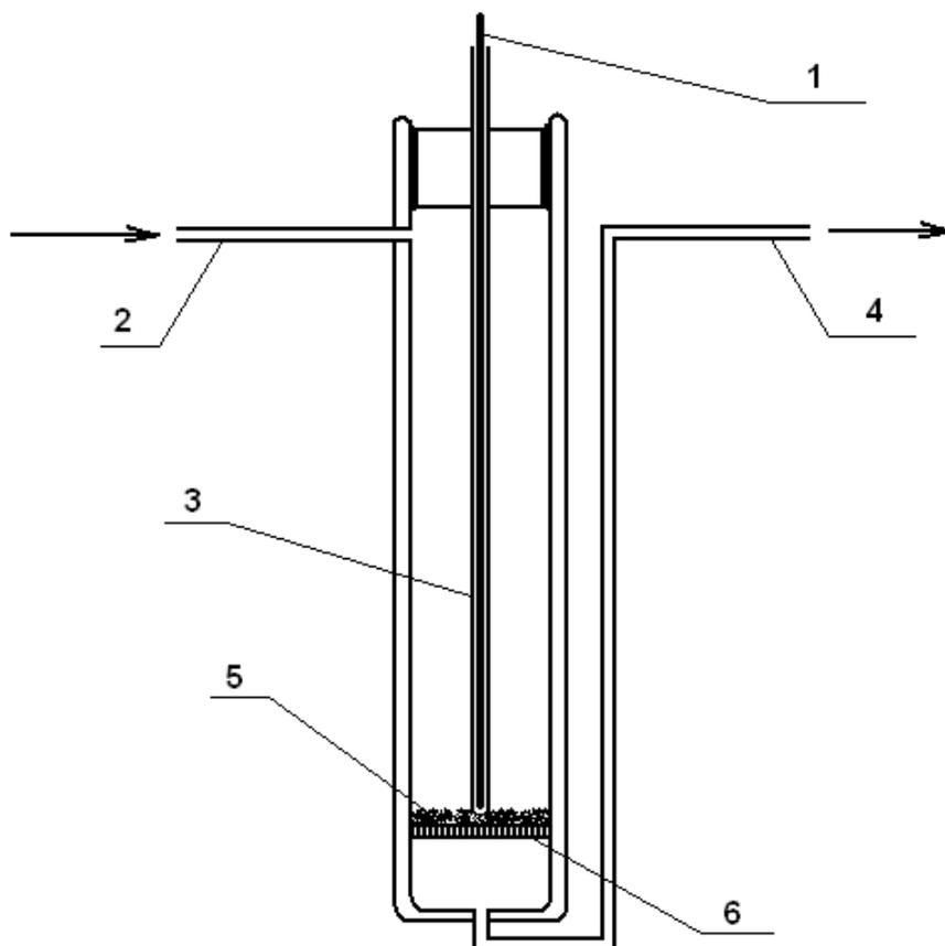
**Figure S1.** Scheme of a quartz reactor ( $d = 6$  mm) of a laboratory flow-through facility for the CO oxidation: thermocouple (1), inlet of the initial gas mixture (2), tube for the thermocouple with the sealed end (3), outlet of the gas mixture that has passed through the catalyst (4), catalyst (5), and grid for the catalyst (6).
