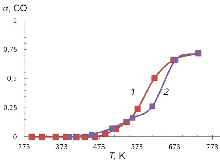
**Figure S2.** CO conversion over the Fe/SiO<sub>2</sub> catalyst depending on the temperature; the Fe concentration was 0.13 wt %; heating (1) and cooling (2).
