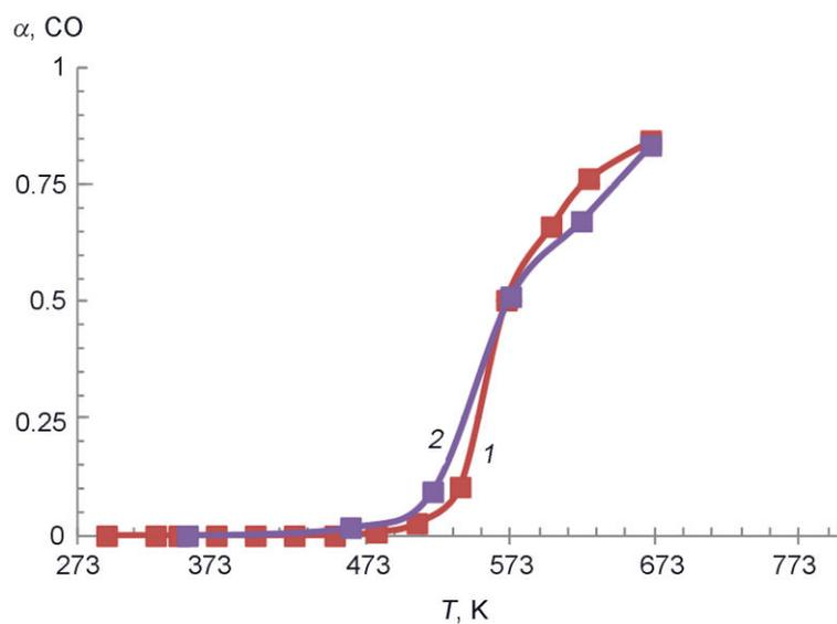
**Figure S3.** CO conversion over the Pd/SiO<sub>2</sub> catalyst depending on the temperature; the Pd concentration was 0.20 wt %; heating (1) and cooling (2).
