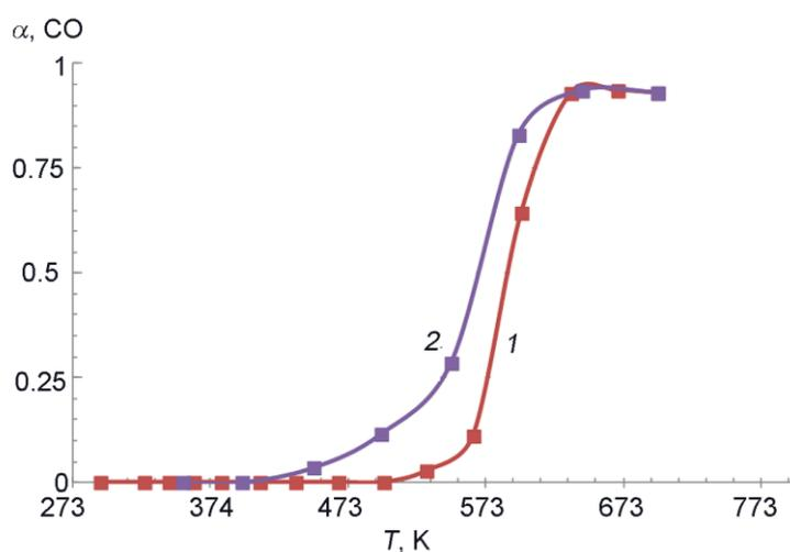
**Figure S4.** CO conversion over the Pd-Fe/SiO<sub>2</sub> catalyst depending on the temperature; the Fe and Pd concentrations were 0.14 and 0.18 wt %, respectively; heating (1) and cooling (2).
