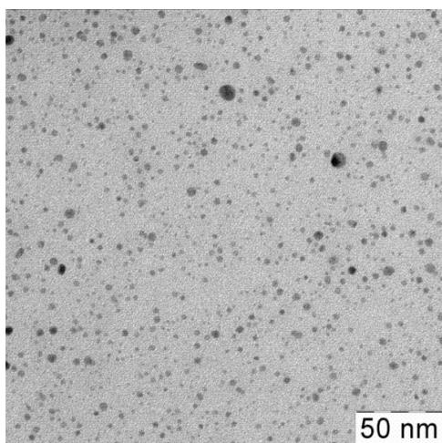
**Figure 1.** TEM micrograph of the  $\text{EMA}/\text{Ag}^0$  particles.
