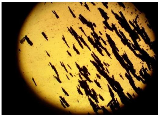
**Figure 3.** Magnetic composite particles in the magnetic field (optical microscopy micrograph ( $\times 10$ )).
