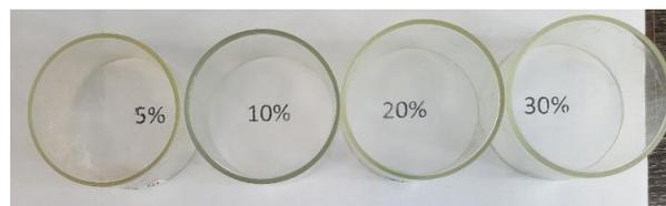
Figure 4. Photographs of the resulting films bearing 5, 10, 20, and 30 wt % of n-PPSQ.
