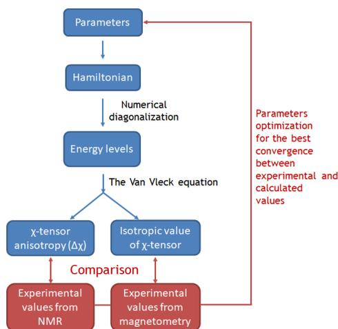
Scheme 2. Algorithm for optimization of the ligand crystal field parameters based on the data of NMR spectroscopy and magnetometry.
