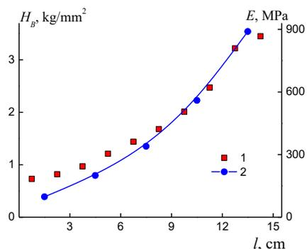
**Figure 5.** Change in the Brinell hardness number at the load of 15 kg and change in the elasticity modulus of the material depending on the macrosample length: 1 – dependence of  $H_B$ , 2 – dependence of  $E$ .
