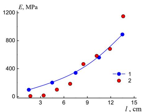
**Figure 3.** Dependence of the elasticity modulus on the length of the gradient material sample: 1 – material obtained on a modified unit; 2 – material obtained on a unit with manual control of the speed of precursor outflow [12].
