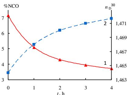
**Figure 7.** Dependences of changes in the mass fraction of the NCO groups (1) and the refractive index (2) on the reaction time during the synthesis of the urethane prepolymer based on PPG-2000 and 2,4-TDI.
