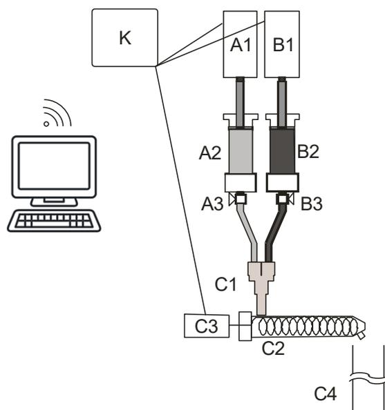
**Figure 8.** Schematic view of a unit for production of gradient polymer materials. A1 and B1 are the electromotors, A2 and B2 are the capacities for compositions, A3 and B3 are the isolation valves, C1 is the chamber of a blending unit, C2 is the dynamic blender, C3 is the electromotor of the blender, C4 is the mold for vertical casting, and K is the control unit.
