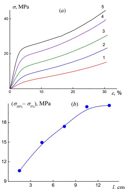
**Figure 1.** Stress–strain curves of the samples (a) cut from sections 1 (1), 3 (2), 5 (3), 7 (4), and 9 (5) and the dependence of the stress difference at 5 and 30% deformation on the macrosample length (b). The location diagram for the considered macrosample zones is presented in Fig. 2.
