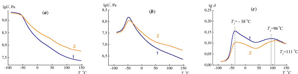
**Figure 6.** Dependences of the storage modulus (a), the loss modulus (b) and the mechanical loss tangent (c) on the temperature. The samples contained zones 1–4 (1) and 5–8 (2).
